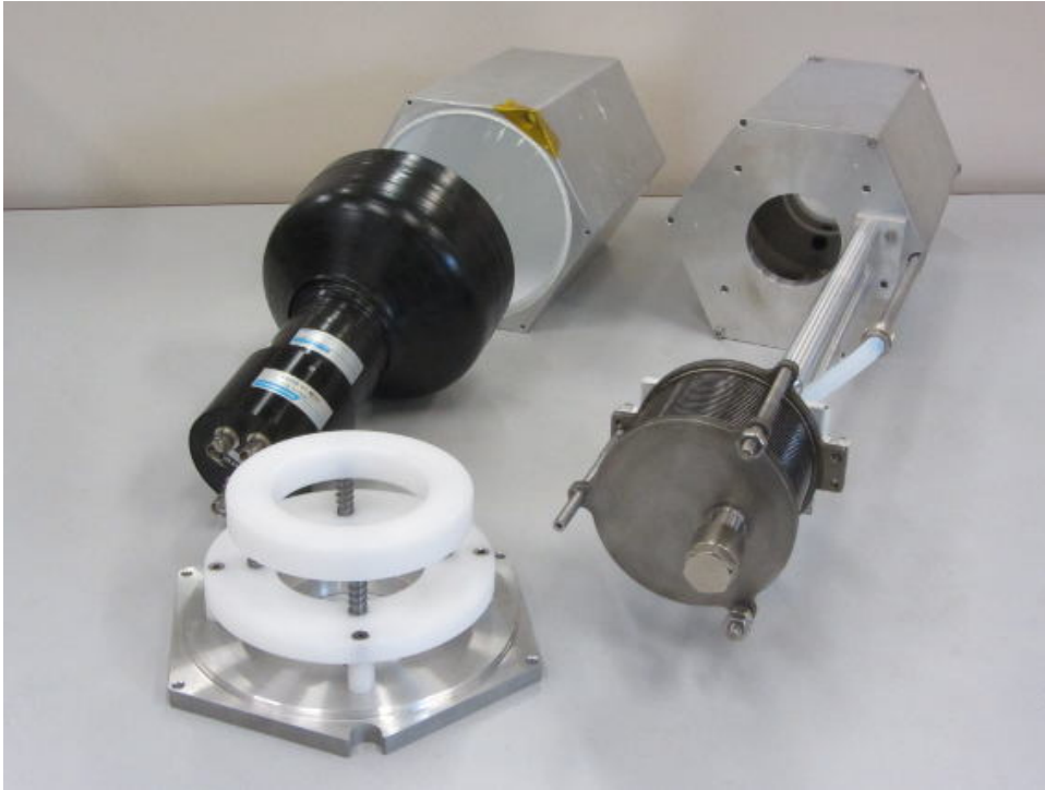
Figure 72: A photograph of the first NEDA prototype detector unit without liquid. Once filled with liquid, the pipe, the bellow and the cell will be bonded together.
