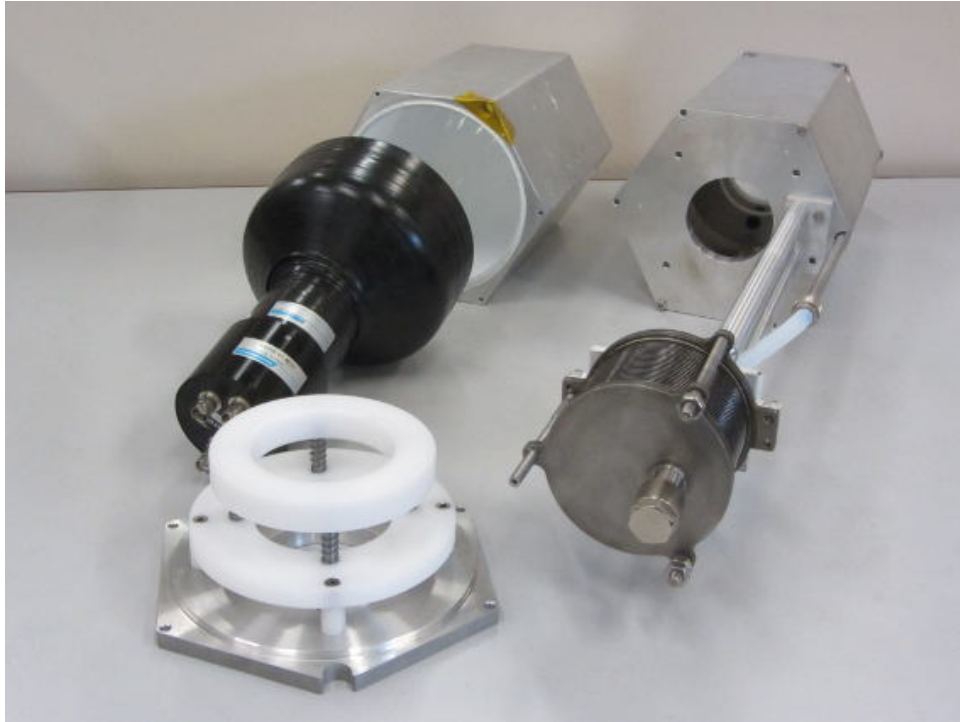
Figure 72: A photograph of the first NEDA prototype detector unit without liquid. Once filled with liquid, the pipe, the bellow and the cell are bonded together.
