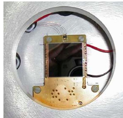
2016 - ... TIMEPIX (Medipix2) 512 x 512 55mm pixels (~1 kHz?)
