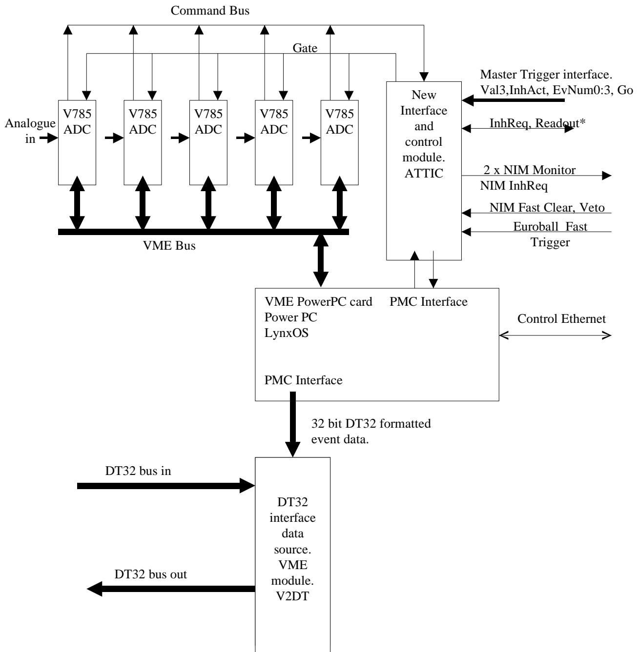
Proposed Readout System for the EUROBALL Neutron Wall
