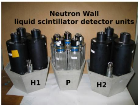
50 closely packed liquid scintillator detectors of three types: H1, H2, P.
